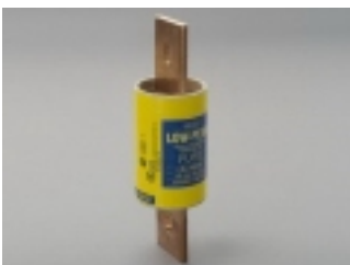
03227 fuse link 400 A, fast acting 600 V AC, 300 V DC
